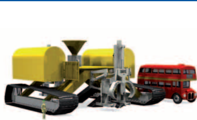
Nowadays thousands of kilometres of cables are laid cross the atlantic. Track plates made from Nylatron GSM are fitted on huge ROV (Remotely Operated Vehicle) trenching machines. These machines operate sub-sea and have the dual function of both digging trenches to enable pipes to be laid, and actually laying the pipes which are then connected to the offshore oil and gas platforms. The material was chosen in preference to the traditional steel mainly because of the significant saving in weight (it typically weighs 1/3 less than steel). However, other advantages are low adhesion (dirt does not build up as it does on steel) and increased traction. (The artists impression gives an indication of the immense scale of these vehicles when compared to a London bus.)
